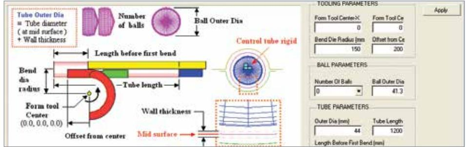
Automated setup for tube bending
