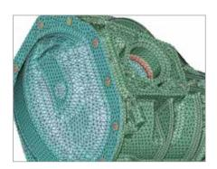
Automated Transmission NVH Analysis from CAD to Vibration Results in 24 hours
