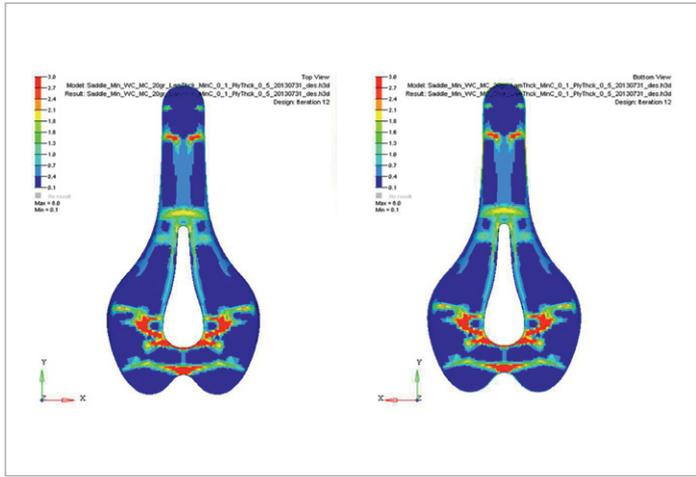
The optimization prior to production (here layer thickness optimization) creates a load efficient and weight minimized component structure
