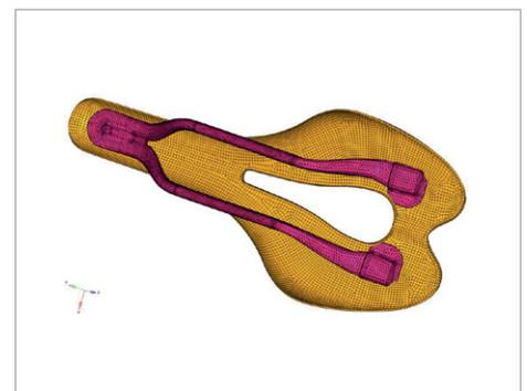
*FE-Model of the bicycle seat – the pilot test object of the process*
