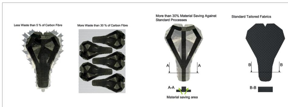
*The FPP-process has very little material waste. Compared to the traditional manufacturing method without optimization, the automated optimization process helped to reduce the material waste by 50 percent*
