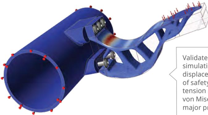
Validate designs using simulation and visualize displacement, factor of safety, percent of yield, tension and compression, von Mises stress, and major principal stress.
